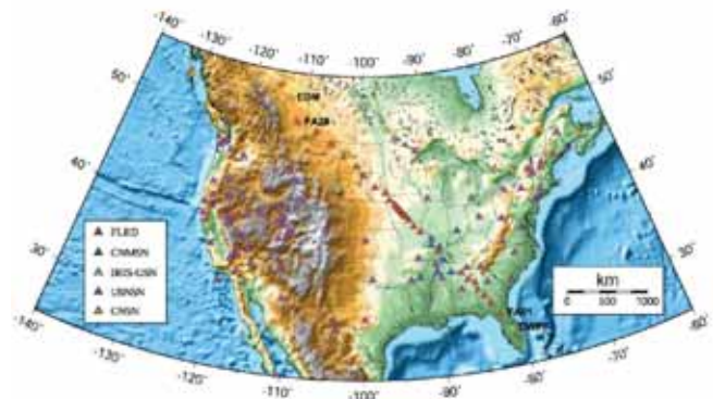
Figure 1. The station locations of the Florida-to-Edmonton (FLED) broadband seismic array.
