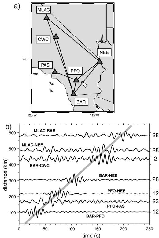
**Figure 3.** (a) Map showing six TERRAScope stations located in California. (b) Stacked cross-correlations of vertical-component short-period (5–30 s) computed from continuous records taken between 03/11/1996 and 04/09/1996. Gray line indicates times corresponding to velocity of 3 km/s. Total durations in days of the noise records available for each pair of stations is indicated on the right side of the plot.
