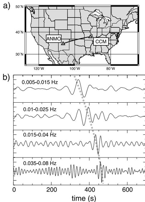
**Figure 1.** (a) Map showing the station location. (b) Cross-correlations of vertical-component records bandpassed with different filters as indicated in top left corners of each frame. Gray dotted line emphasizes the dispersion of the emerging signal.
