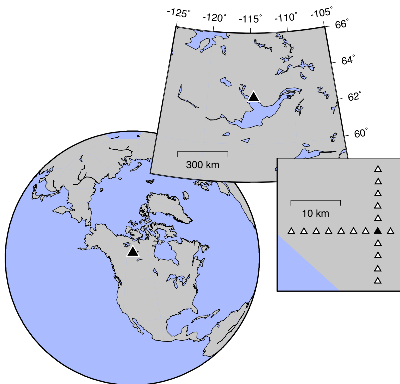
Figure 1. Geometry and location of the Yellowknife seismic array (YKA). The darkened triangle is the reference element of the array. The large body of water south of the array is the Great Slave Lake.
